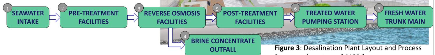
Figure 3: Desalination Plant Layout and Process Summary (courtesy of AJCJV)
